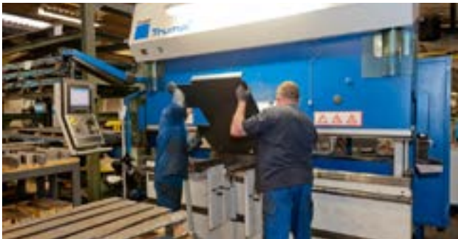
Computer assisted steel plate bending
