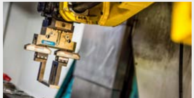
Part picking by robot
