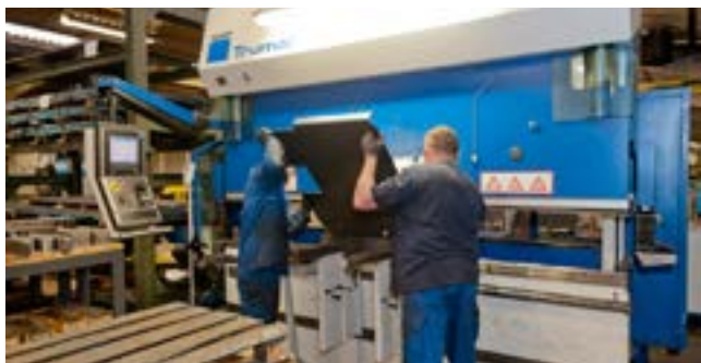
Computer assisted steel plate bending
