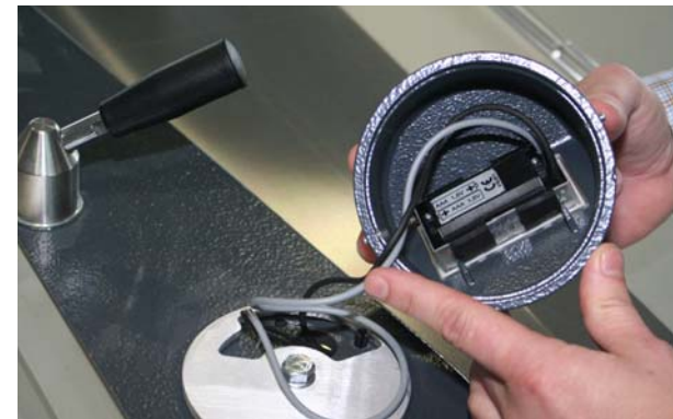
Fig. 6-138: Remove the housing with the display unit
