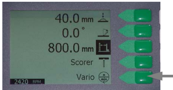
Fig. 6-35: Setting the rotational speed
