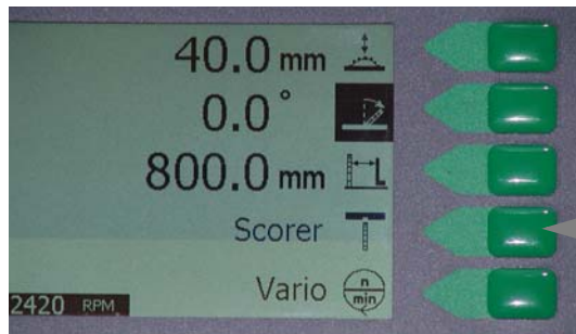
Fig. 6-37: Adjusting the scorer
