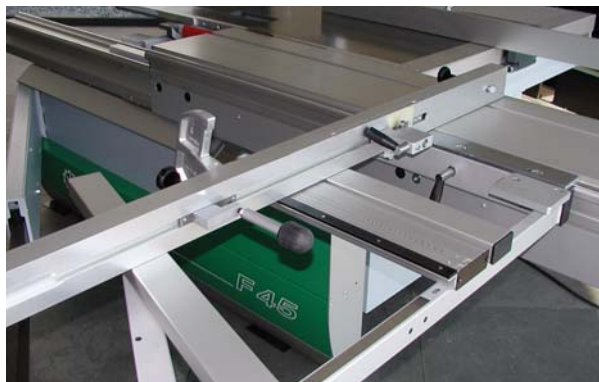
Fig. 5-12: Installing the WGA
