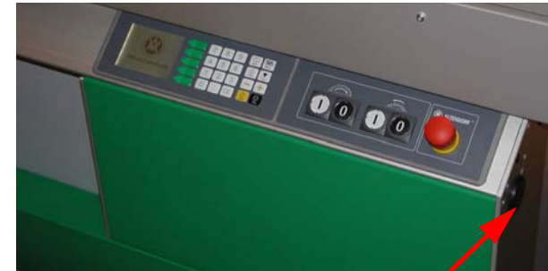
Fig. 6-52: USB port on the machine frame
