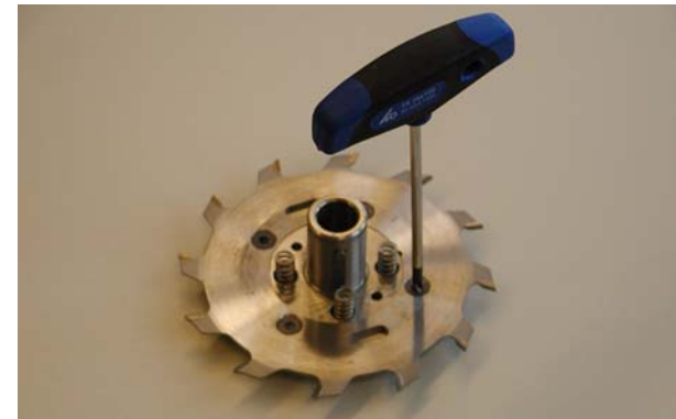
Fig. 6-117: RAPIDO Plus, fitting saw blade
