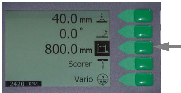
Fig. 6-34: Rip fence adjustment
