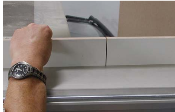
Fig. 5-54: Checking the 0° -setting
