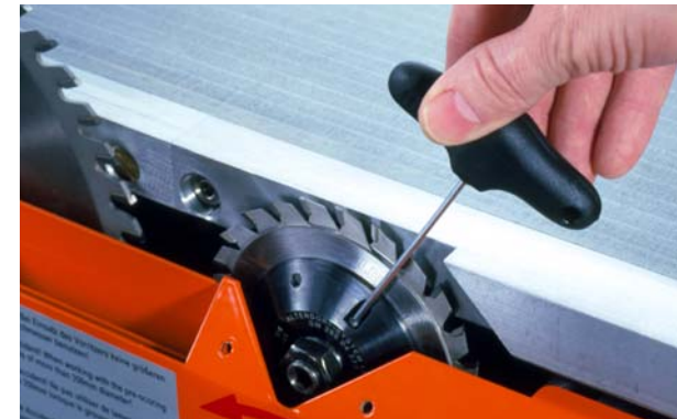
Fig. 6-112: Releasing the clamping screw
