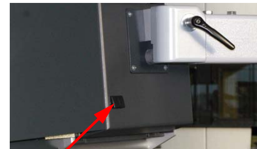
Fig. 6-53: USB port on the eye-level operating panel
