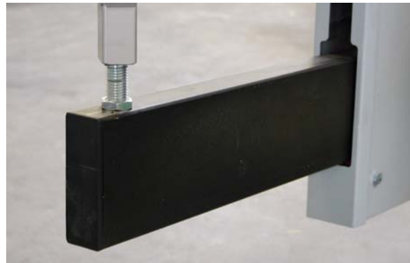
Fig. 5-49: Adjusting the cross-slide height
