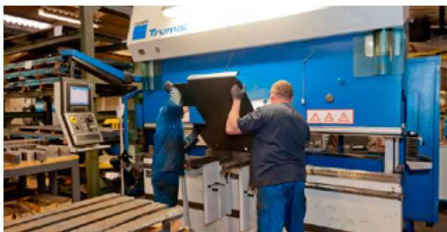
Computer assisted steel plate bending
