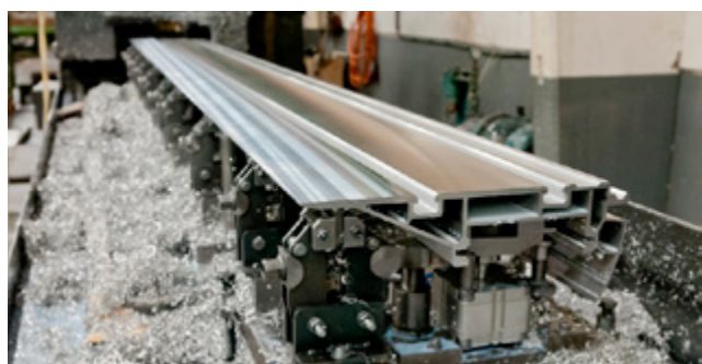
Milling of sliding table surface
