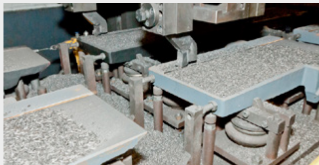
Surface scraping of cast iron table
