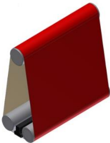
Single Sanding Head installed with Roller – Pad configuration.
