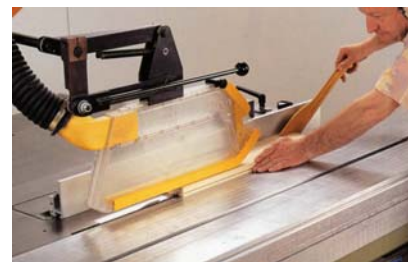
Protective equipment and handling for cutting rebates
