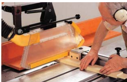
Safety equipment and handling for cross-grain cutting of pins
