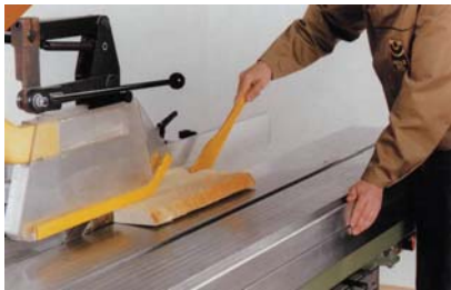
Cut narrow workpieces with a push stick
