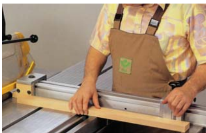
Cutting narrow workpieces to length with the cross fence
