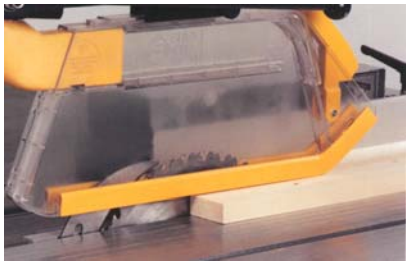
Adjust the guard to the workpiece thickness or lower it to the machine table
