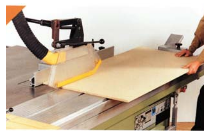
Safety equipment and handling for insert cutting
