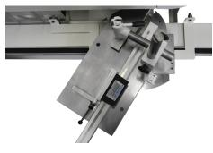
The table can be swivelled 60° in two directions. The working area of the table does not change.
