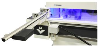
The automatic length fence allows the operator to size workpieces to length, and the large swiveling backstop allows for the sizing of two pieces at the same time.
