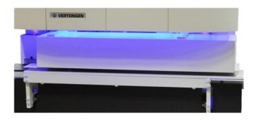
The belt feeding device can transport parts with a minimum length of 100mm / 4"
