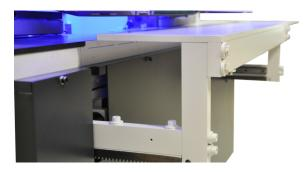
The automatic outside fence allows the operator to change-over in a short time between parts of different widths.
