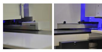
The infeed-unit aligns the workpiece accurately under the main belt while the outfeed-unit delivers finished parts to the operator.
