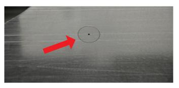
Air nozzles in the steel table create an air cushion between the workpiece and the machine surface for better through-feed.
