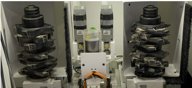
Spindles of 300 mm with Prolock both individual horizontal and vertical cnc-positioned.
