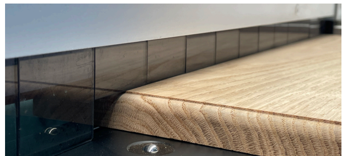
The safety screen will cover the total width of the table and activate before clamping.
