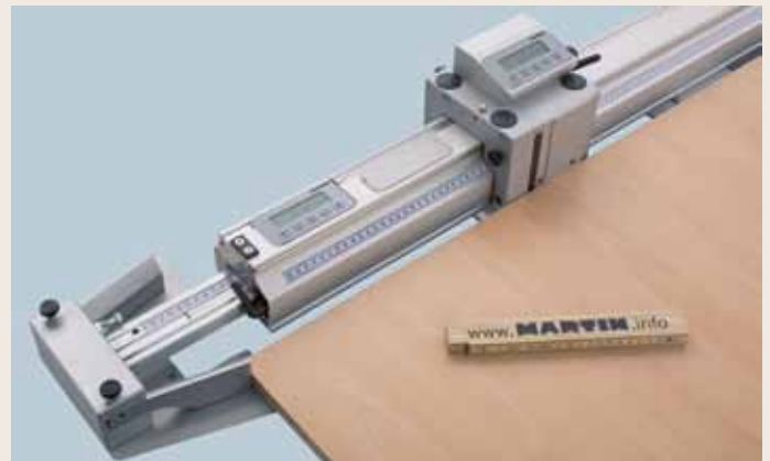
T6542 digital 2-point cross-cut fence
