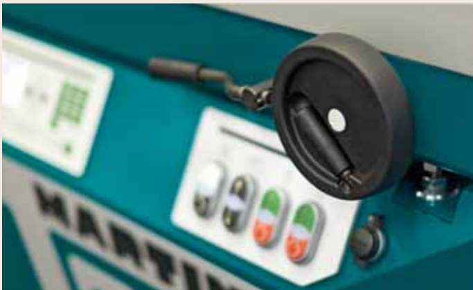
T6589 hand-wheel adjustment of the rip fence
