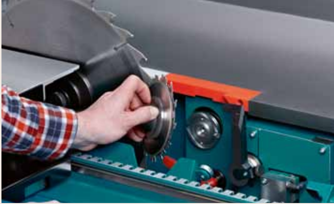
T6523 electrically adjustable 3-axis scoring saw
