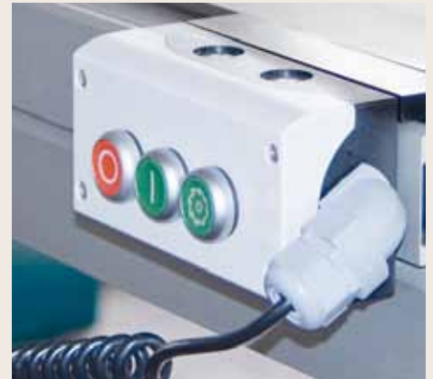
T6577 ON/OFF switch on the sliding-table
