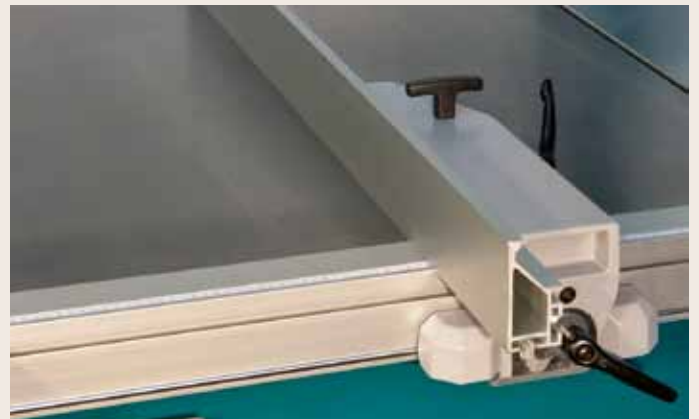
T6590 motorized positioning of the rip fence
