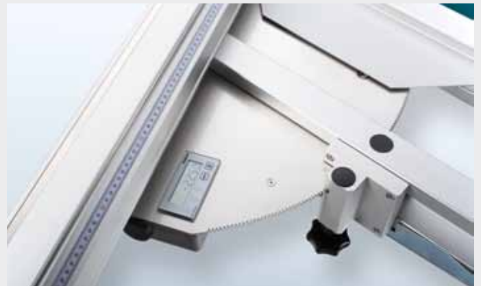
[4] T6535 Miter cross cut table
